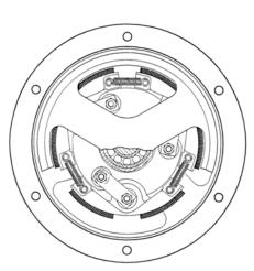
.343 DIA. (6) PLACES EQUALLY SPACED ON 8.70 DIA. B.C.
