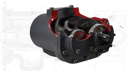
Solidly built, compact HILCO® starters can provide starts within 30 to 40 seconds using pressurized air or natural gas actuation, plus they are capable of extended purge times of five minutes or longer. These starters are field-proven to provide high torque on demand for cranking gas turbine and reciprocating engines.
