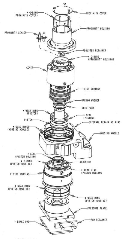
ONE MODULE SHOWN • RECOMMENDED SPARE PART (SEALS, O-RINGS AND WEAR RINGS AVAILABLE AS A KIT)
