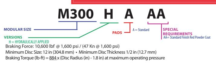
Brake Weight: 46 lb (20.8 kg) Brake Path: 4.125 in (104 mm) Friction Pad Area: 10.9 in<sup>2</sup> [70 cm<sup>2</sup>] (Each Pad) Oil Volume: .25 in.<sup>3</sup>
