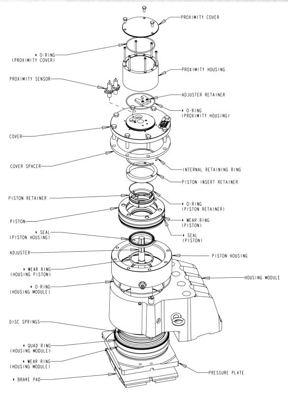
ONE MODULE SHOWN \* RECOMMENDED SPARE PART (SEALS, O-RINGS AND WEAR RINGS AVAILABLE AS A KIT)
