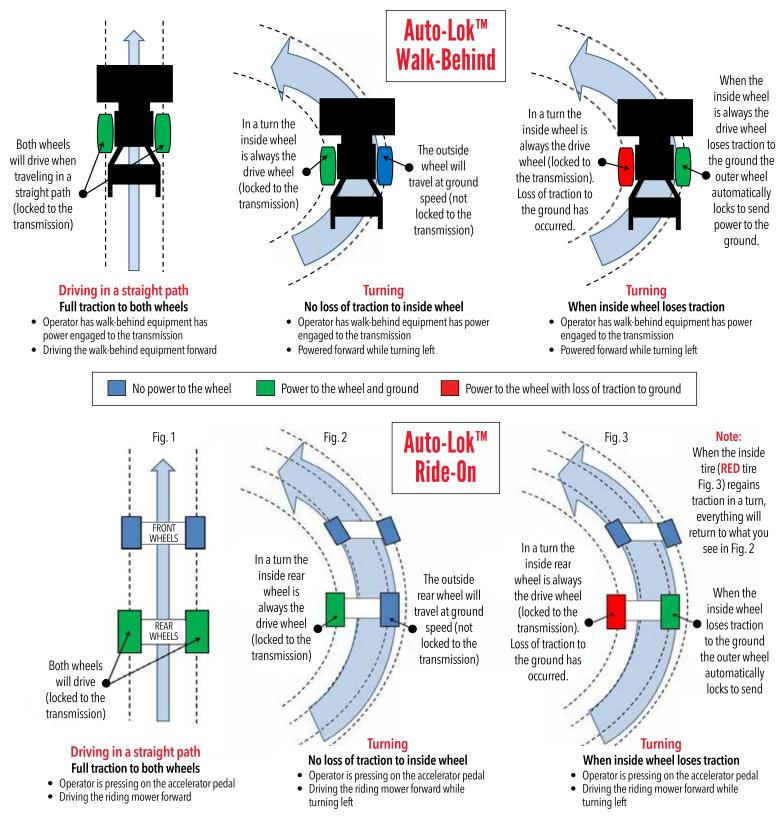
When wheel's speed exceeds the speed of the clutch housing, the cage will shift the rolls to the opposite engagement angle, allowing the machine to descend down the gradient at the speed of the transmission.
