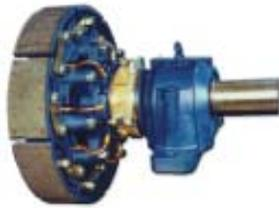
This system combines the advantages of a link clutch with the additional features of engagement/disengagement at any speed. It also provides overload protection by disengaging immediately on heavy overload, protecting the clutch and the rest of the transmission equipment.
