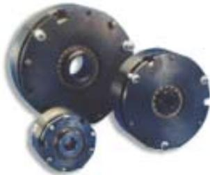
Designed for maximum flexibility and long, dependable service, our electric brake is electromagnetically released when voltage is applied and spring-engaged when current is interrupted.
